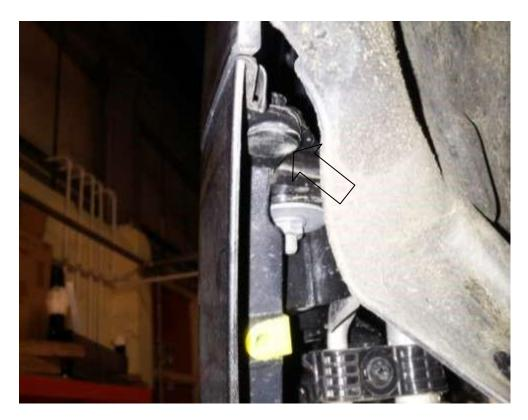
10. From underneath the vehicle reach inside the bumper and disconnect the wiring to both fog lights (if fitted to the vehicle).
