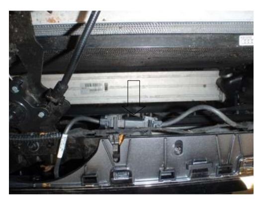
1. Using a T30 Torx, extension short bar and suitable small ratchet (ideally ¼" drive) undo 1x bolt located underneath headlight on the inside of the wing on both sides. This is very awkward, as you cannot see the bolt you are trying to undo.
