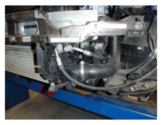
15. Unclip the intercooler top mounts on both sides, pull airguide to oneside, and lift the intercooler off its lower mounts.
