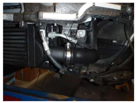
18. Using the silicone elbow, aluminium coupler and hose clamps provided connect the turbo outlet hose to the intercooler. Do not fully tighten the hose clamps until all parts have been installed.
