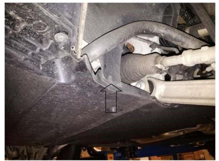
6. Using a T25 Torx driver remove 3x screws inside the edge of the arch liner and 2x T25 behind the wheel on both sides of the vehicle.
