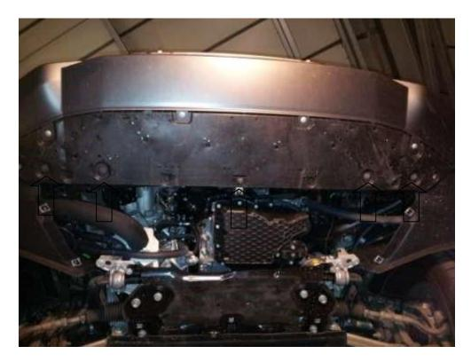
8. Using a T25 Torx Driver undo 1x screw on both sides of the vehicle.
