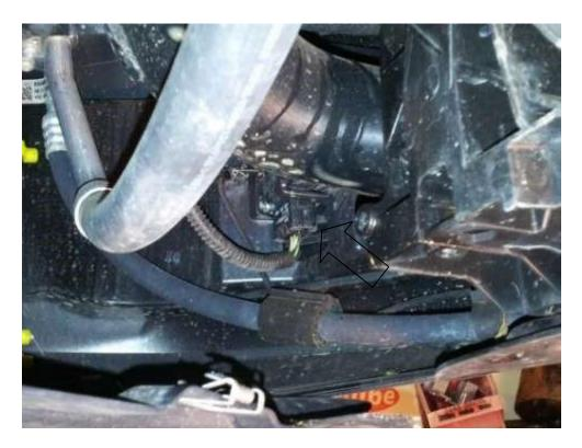
11. Using a T30 Torx driver undo the x4 screws.
