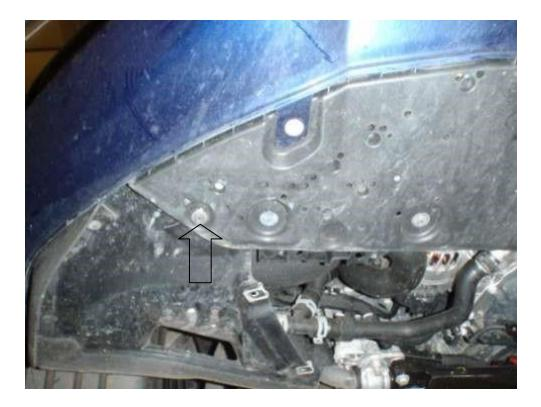
9. Carefully pull the arch liner to one side. Using a panel-clip removal tool or flat blade screwdriver remove the vertical plastic clip, if necessary lubricate the plastic clip with silicone spray or similar.
