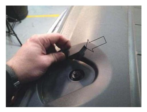
4. Starting on the front edge carefully pull the plastic cover upwards to release it, then slide the panel forwards to remove it.
